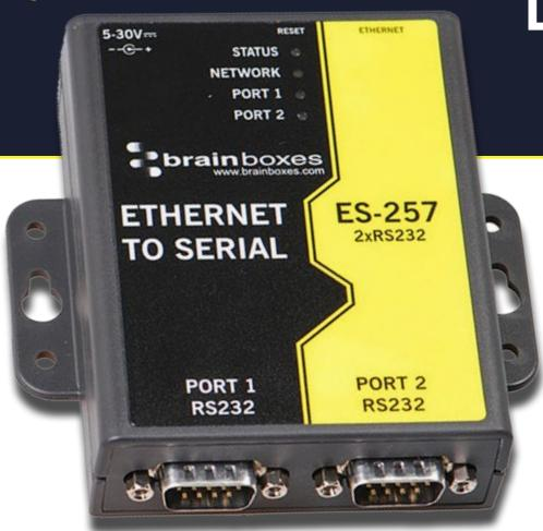
Install Virtual Com ports, communicate over TCP or telnet or use the software APIs for Visual Basics, C# & more
