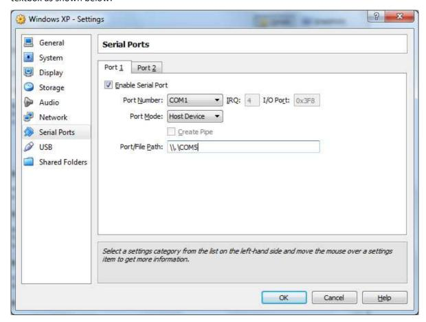
Please note that for this demonstration I have installed Brainboxes **US-101** product in the Host Operating System and this is installed as "**COM5**" in my machine as shown below:
