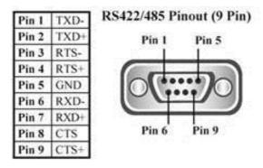
You will need to either short pins 1+6 and 2+7 or construct a Half-Duplex cable with those pins shorted.
