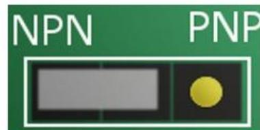
NPN or PNP jumper position should be changed depending on the type of sensor/input.
