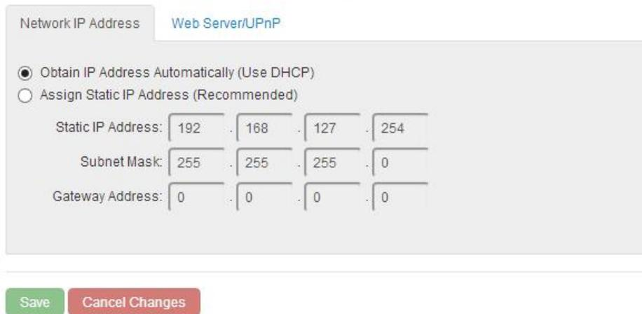
In the Network IP Address tab you can select whether the device is using DHCP or a static IP address which you specify. By default the ED device is set to use DHCP to obtain an IP address automatically. If there is no DHCP server present, after 60 seconds the device will switch to a static IP address of 192.168.127.254.
