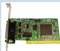
UC-083 uPCI 4xRS232 Opto Isolated TX RX GND CTS RTS
