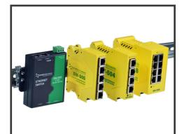
Integral DIN mount and slim design provides Ethernet connection to multiple devices
