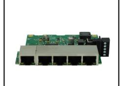
Embedded format, takes up minimal space, with mounting holes connected to Functional Earth
