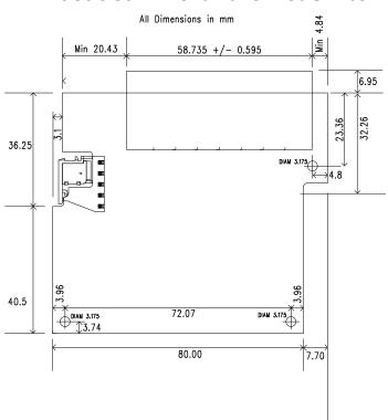
5 position 3.5mm pitch socket compatible with Euroblock pluggable terminal block connectors
