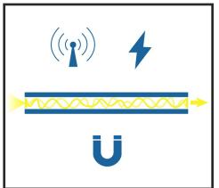
Fibre cables are immune to any electrical/magnetic interference, and require no cumbersome isolation devices to guard against high EMI/RFI or lightning strikes
