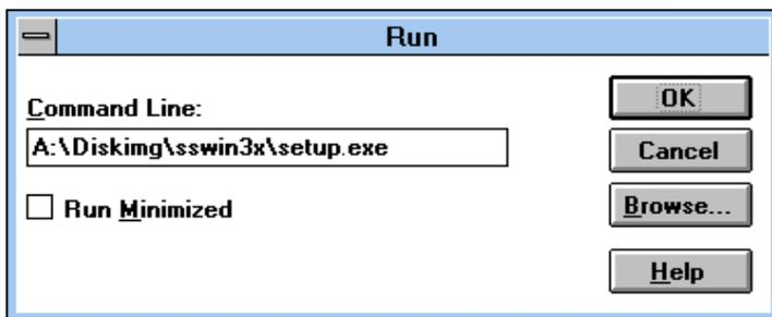
To install the software from the supplied disk, insert the disk from Windows **Program Manager's** File menu choose "Run" and in the Command Line entry window type <drive:>\disking\sswin3x\setup.exe (where <drive:> is the path to the CDROM drive containing the installation disk).
