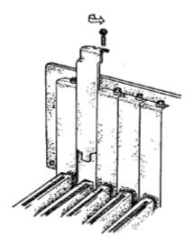
Choose an empty expansion slot. This Card will fit into one of the white PCI slots on your motherboad. Remove the blanking cover protecting the slot on the PC back panel. KEEP the blanking cover screw safely for later.
