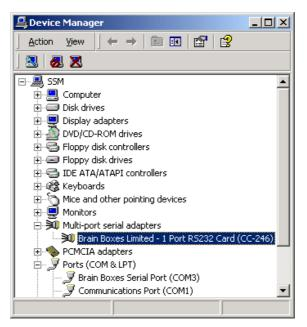
By double-clicking on the **Multi-port serial adapters** label you will reveal any cards that you have installed. Double-click on the **PCI 1 Port RS232 Card** label.
