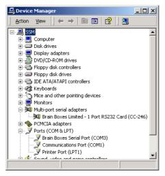
The PCI 1 port RS232 card will appear under **Multi-port serial adapters** . Also, a Brain Boxes Serial Port will appear under **Ports (COM & LPT)**.
