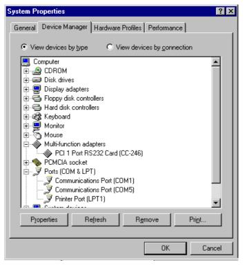
When the "**Device Manager**" is viewed the PCI 1 port RS232 card will appear under the "**Multi-function adapters**" branch. Also, a Communications Port will appear under the "**Ports (COM & LPT) branch**".
