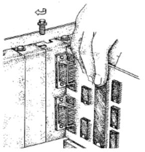
Now insert the card in the slot. Be careful to ensure that the gold plated pcb fingers fits neatly into the I/O expansion connector. Press down firmly but evenly on the top of the card.
