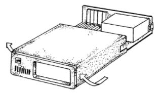
Next, remove the PC's cover by sliding it forward and up. It usually helps to disconnect the keyboard from the PC since it tends to get in the way when the case is removed.
