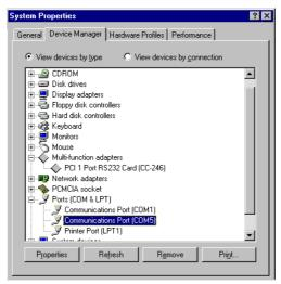
Double-clicking on the **Ports (COM & LPT)** label you will reveal a list of ports installed on your machine. Click on the port you wish to configure to configure to highlight it, then click on the **Properties** button.
