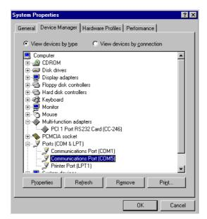
Double-clicking on the **Ports (COM & LPT)** label you will reveal a list of ports installed on your machine. Click on the port you wish to configure to configure to highlight it, then click on the **Properties** button.
