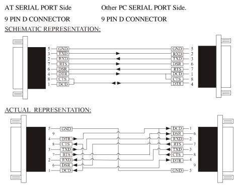
Suppose we want to connect the AT style 9 pin D Serial Port to the serial port of another IBM PC.
