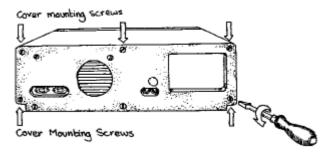
Then using a screwdriver, remove the cover mounting screws on the back panel of the PC system unit.
