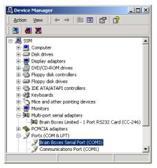
Double-clicking on the **Ports (COM & LPT)** label you will reveal a list of ports installed on your machine. Double-click on the port you wish to configure.
