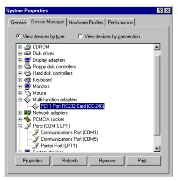
By double-clicking on the **Multi-function adapters** label you will reveal any cards that you have installed. Click on the **PCI 1 Port RS232 Card** label to highlight it, then click on the Properties button
