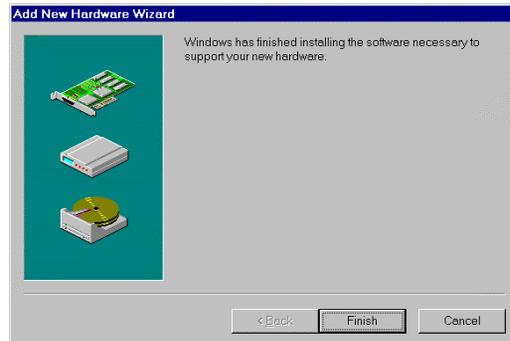
You will then be asked if you wish to re-boot the system. Since the multiport card will now need to be installed, select yes. Turn the PC off and insert the multiport card as described in chapter 3, making changes to settings on the card as necessary. Restart the computer and allow Windows 95 to load normally. Upon loading it will then "detect" each of the ports on the Lynx card individually and install them, in a similar manner to that of a Plug and Play card.
