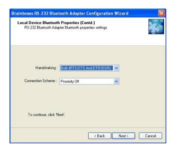
The Handshaking Options and Proximity Mode of the device are configurable on this screen.
