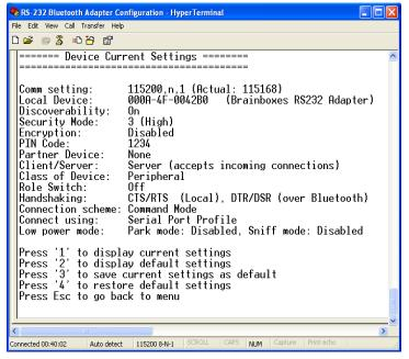
The first screen that displays shows the current state of the adapter's settings.
