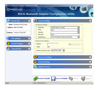
Add the address of your remote device into the "Partner Device Settings" Section in the "Address" field.
