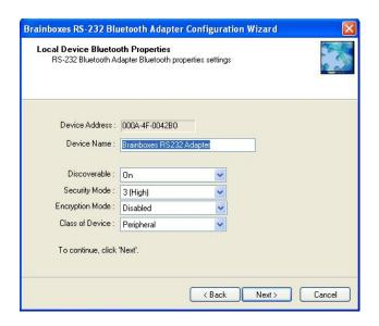
The Standard Bluetooth Properties of the Adapter are presented next, along with the MAC address of the device. This is not user changeable.
