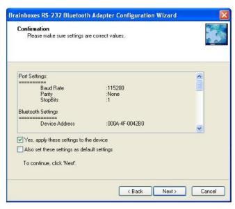
Finally the user will be able to view all the settings which will be applied to the Adapter, and confirm whether they wish to apply them to the device.
