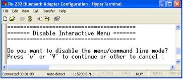
Selecting 'y' or 'Y' from this menu means that no further interaction with the menu will be possible until the device has been completely reset to it's factory defaults by performing a "long" reset from the reset button.
