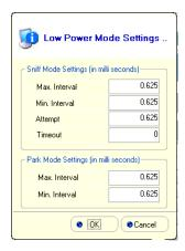
The settings used for the low power modes can be changed to suit whatever the application is that the devices are being used for. Increasing interval times will reduce the power usage, but will also increase the response time of the adapter's as they are "out of action" for much longer.
