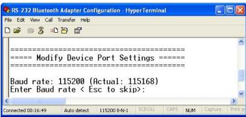
The user is first prompted to change the Baud Rate. The current setting is shown. To change the baud rate, just type the rate you want to use and press <enter>. The Adapter will accept any number you type, but will set the baud rate to the one that's closest to what it can actually achieve.
