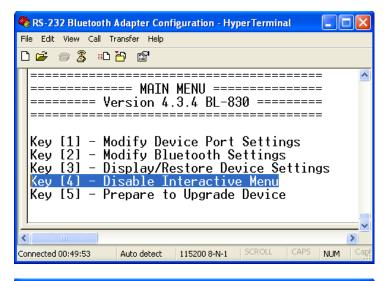
Some RS232 devices (GPS devices for example) emit a continuous stream of data regardless of whether a cable is connected. When no Bluetooth connection exists, this data can actually appear as commands to the menu and change settings that render the Adapter inoperable. Disabling the menu, stops the Adapter being unwontedly reconfigured in this manner.
