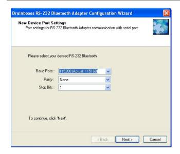
This Screen will allow you to change the RS-232 Port settings for communication to the Adapter.
