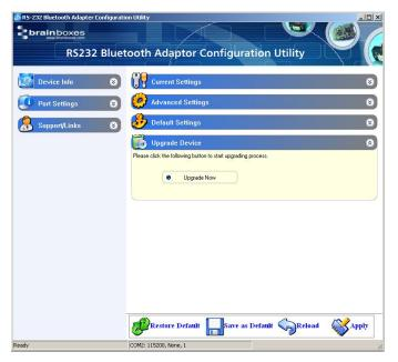
The "Upgrade" section is a new feature that allows the user to upgrade the adapter firmware using a simple upgrade wizard.
