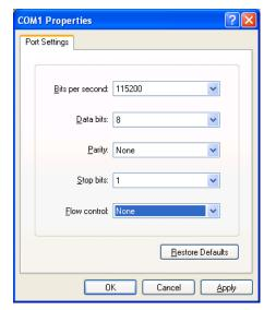
Select the communications parameters that your device is configured to. In this example we have used the factory defaults normally applied. If you have previously reconfigured these values, then you will need to make sure the settings here match those you have configured to device to be.
