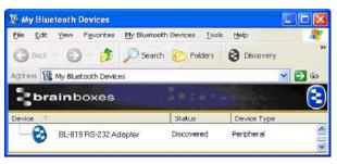
Open the "My Bluetooth Devices" window and click the discovery button to discovering the Adapter using the Brainboxes Bluetooth Windows software. This sets the software to display all the Bluetooth devices it can find "in range".
