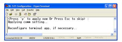
If you have changed any communications parameters, and wish to continue to access the configuration menu, you will need to update your terminal applications settings. The easiest method of performing this in HyperTerminal is to close and re-start the application, setting the new parameters during the initial application configuration.
