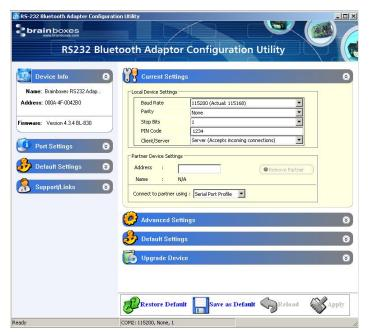
The Current Settings section is broken down into two sections; Local Device Settings and Partner Device Settings. Each field will be discussed further below.
