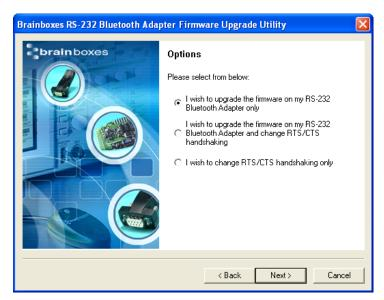
Three options are presented to the user with the choice or either just upgrading the firmware, upgrading the firmware and changing the RTS/CTS handshaking setting or just changing the RTS/CTS handshaking setting.
