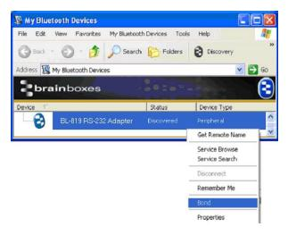
This is where you must "Bond" or "Pair" with the device. This is a feature of Bluetooth, which allows secure communications to take place. It is also used to stop other devices from performing unauthorised connections.
