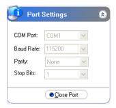
The Port Settings section displays the current used port settings for the connected Adapter i.e. the port settings that were used to open and access the device. This includes the current COM port, Baud Rate, Parity and Stop Rits
