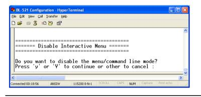
Some RS232 devices (GPS devices for example) emit a continuous stream of data regardless of whether a cable is connected. When no Bluetooth connection exists, this data can actually appear as commands to the menu and change settings that render the converter inoperable. Disabling the menu, stops the converter being unwontedly reconfigured in this manner.
