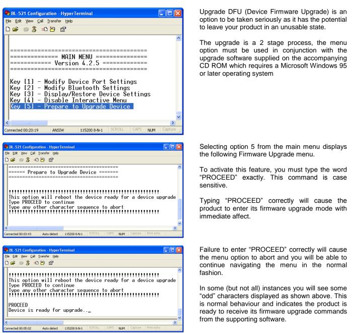
At this point, you will no longer be able to interact with the menu, nor will you be able to use the product as advertised. ONLY the supporting software can restore this setting. Neither a power reset nor any combination of presses of the reset button will restore normal operation to the product. It is now permanently in a state to upgrade the firmware.
