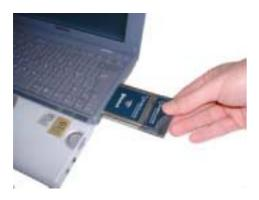
Insert the Bluetooth PC Card into a free PC Card slot
