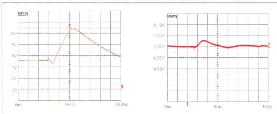
Figure 3. Output voltages during the connection process, left without protective function, right with protective function (Maxpower)
