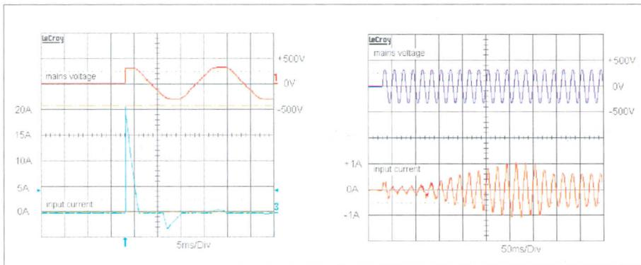
Figure 2. Inrush current behaviour, left conventional, right Maxpower
