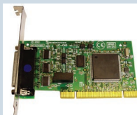
UC-072 uPCI 4xRS232 Opto Isolated TX RX GND
