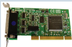
UC-072 uPCI 4xRS232 Opto Isolated TX RX GND
