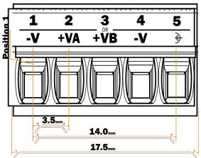
5 position 3.5mm pitch socket compatible with Euroblock pluggable terminal block connectors
