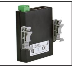
Integral wall mount option can be used with MK-048 clips to allow DIN rail mounting
