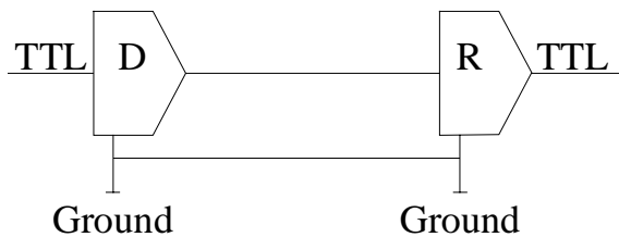
Figure 4-1. RS232 Point To Point Connection.
