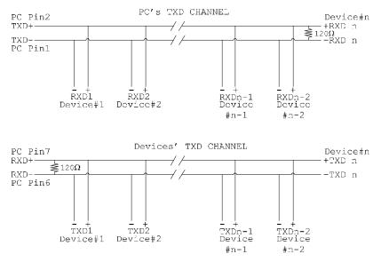
**Note:** The receiver end of MAIN line terminated in characteristic impedance, stubs off the main not terminated.
