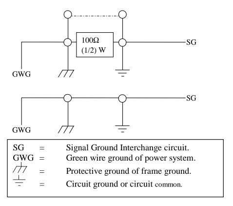
Configuration A) The circuit common of the equipment is connected to protective ground, at one point only by a  $100 \Omega$ ,  $\pm 20\%$  resistor with a power dissipation rating of 1/2W. An additional provision may be made for the resistor to be bypassed with a strap to connect signal common and protective ground directly together when specific installation conditions necessitate.
