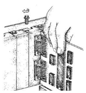
Now insert the card in the slot. Be careful to ensure that the gold plated pcb fingers fits neatly into the I/O expansion connector. Press down firmly but evenly on the top of the card.
