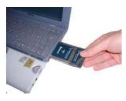
Insert the Bluetooth PC Card into a free PC Card slot. The following screen appears -
